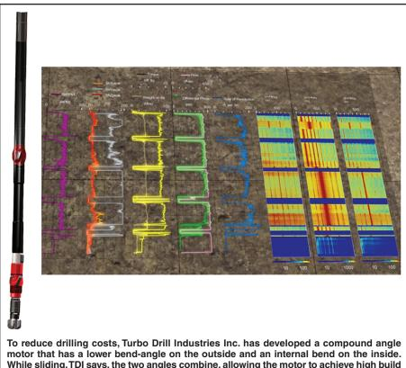
To reduce drilling costs, Turbo Drill industries inc. has developed a compound angle motor that has a lower bend-angle on the outside and an internal bend on the inside. While sliding, TDI says, the two angles combine, allowing the motor to achieve high build rates in the curve. It is embedded with sensors that gather shock, vibration, rpm and temperature data to help pinpoint drilling dysfunctions, TDI adds.
